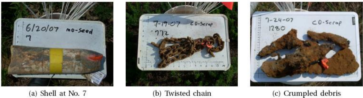
Figure 29: a) Unexploded shell from Cell No. 7 and (b,c) the two false alarms obtained by the SVM classifier using k and Q(t_{15})/Q(t_1) as discriminators.
