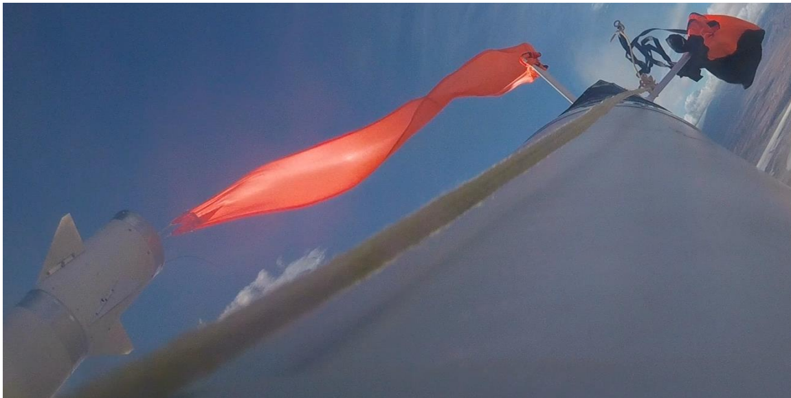
Figure 33. Drag Equipment / Rear Fin Interaction
