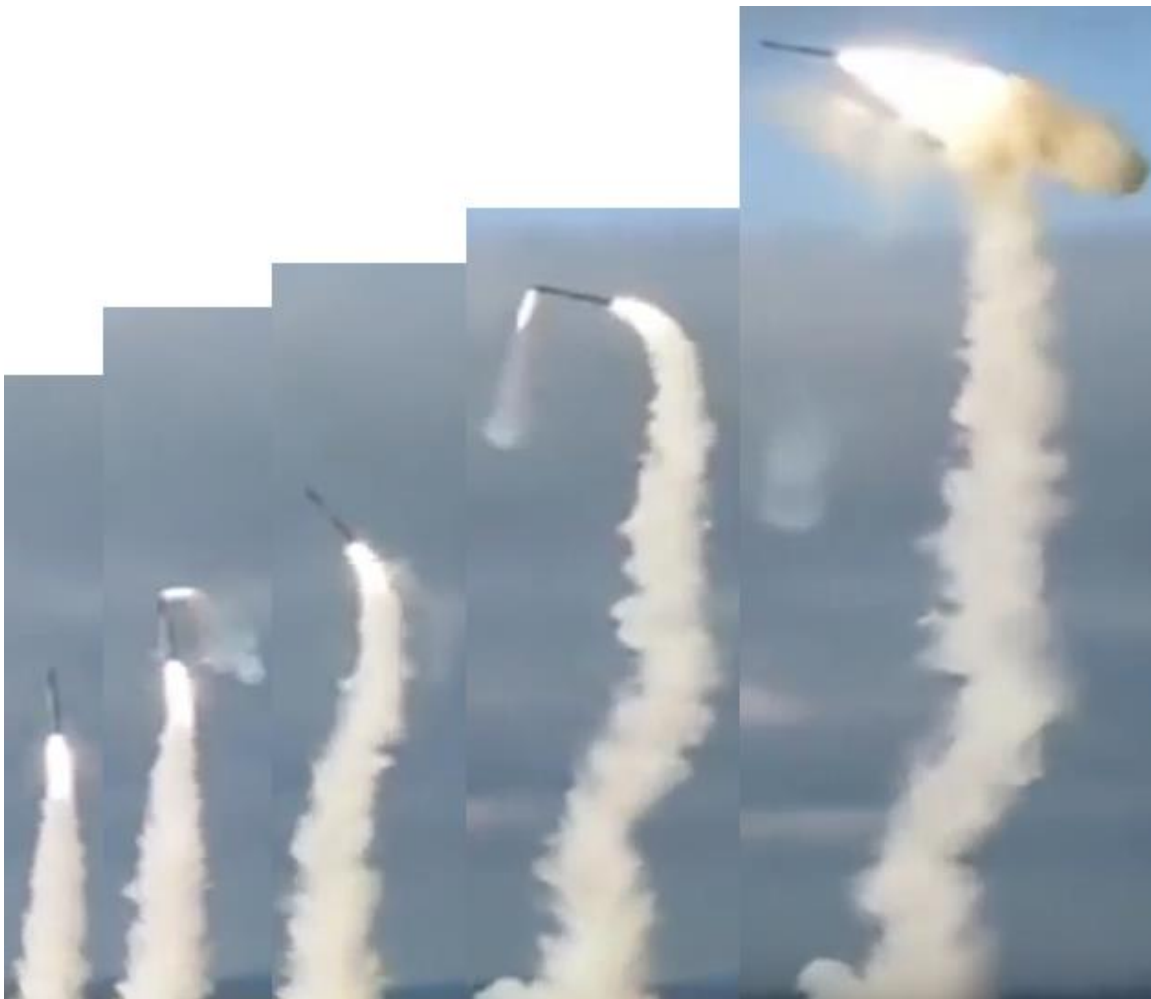
Figure 8. Example of Lateral Thruster Employment. Source: [35].
