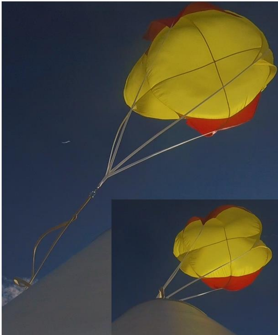
Figure 34. Parachute Failure; Inset is the Video Frame Prior to the Frame Shown Large
