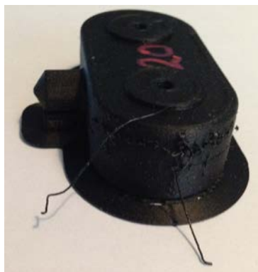
Figure 22. Part with Material Splatter
