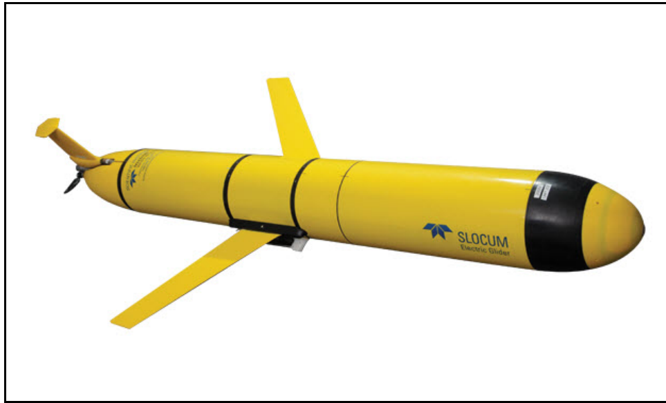
Figure 4. Slocum Glider (Available at: https://www.sequoiasci.com/about/news/lisst-glider-development/ ).
