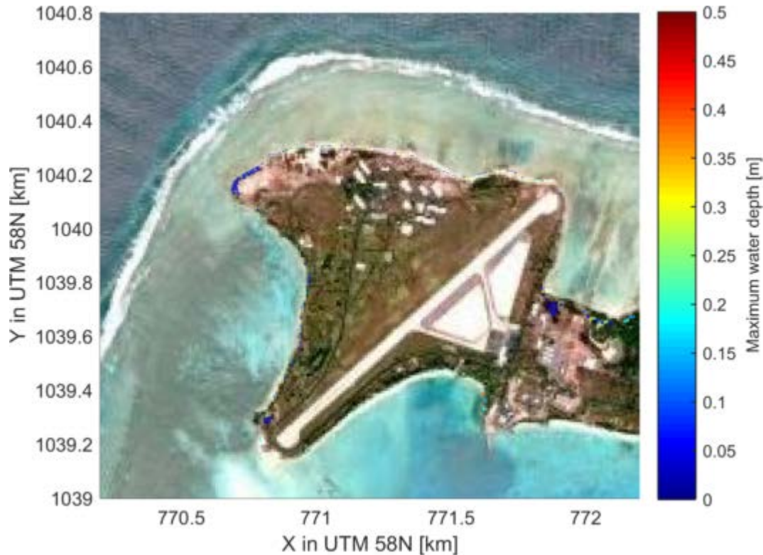
Figure 43. Map of modeled wave-driven flooding depth for the calibrated 2D XBeach model during the March 2014 overwash event on Roi-Namur. The color bar denotes the maximum water depth on the island during the March 2014 overwash event.
