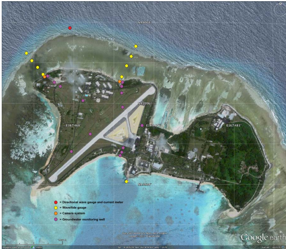
Figure 4. Photograph of Roi-Namur showing location of instrumentation deployed on Roi for this study. The colored circles represent the following: red = directional wave/tide gauge; yellow = non-directional wave/tide gauges; orange = time-lapse camera systems; purple = groundwater wells.
