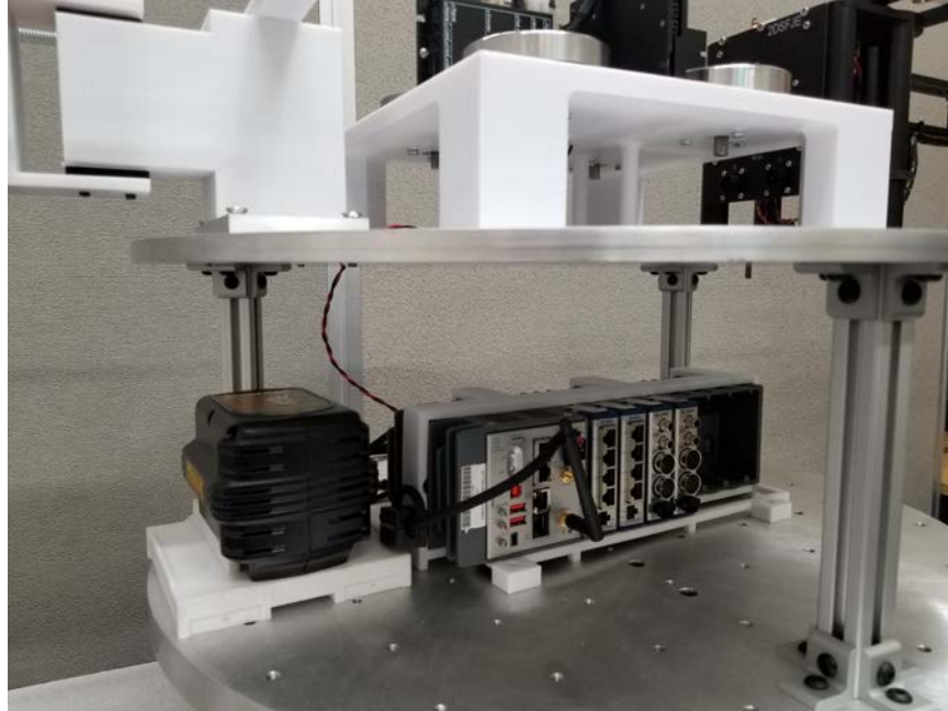
Figure 19. Battery connected to cRIO and reaction wheel array
