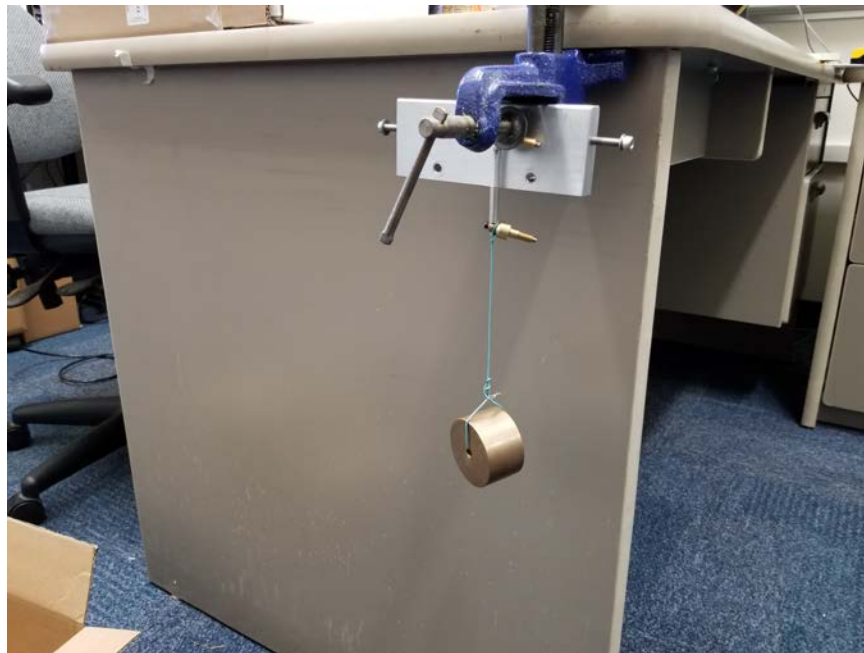
Figure 22. Measuring the 2DOFSFJ spring constants
