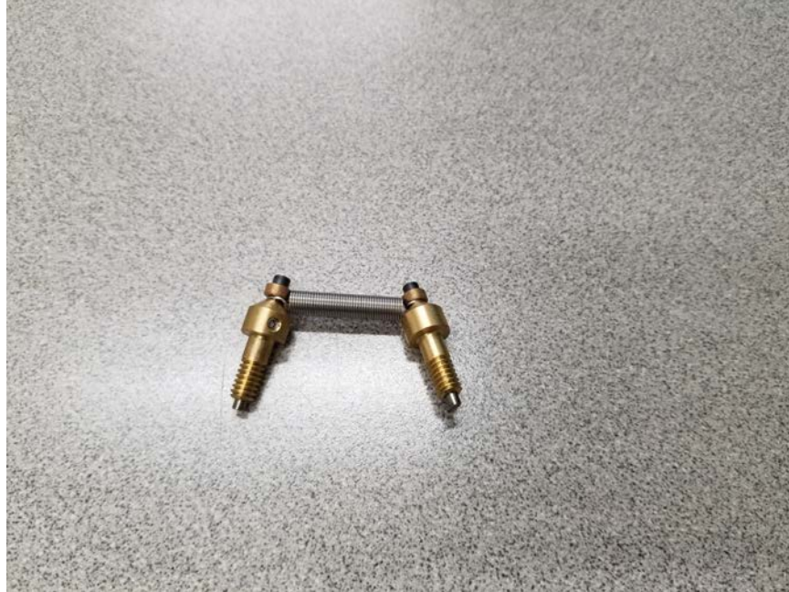
Figure 23. Spring with brass connectors
