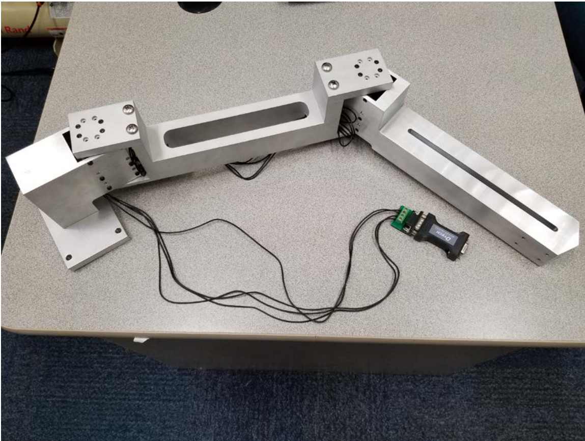
Figure 16. Two-link rigid robotic arm designed and manufactured at NPS
