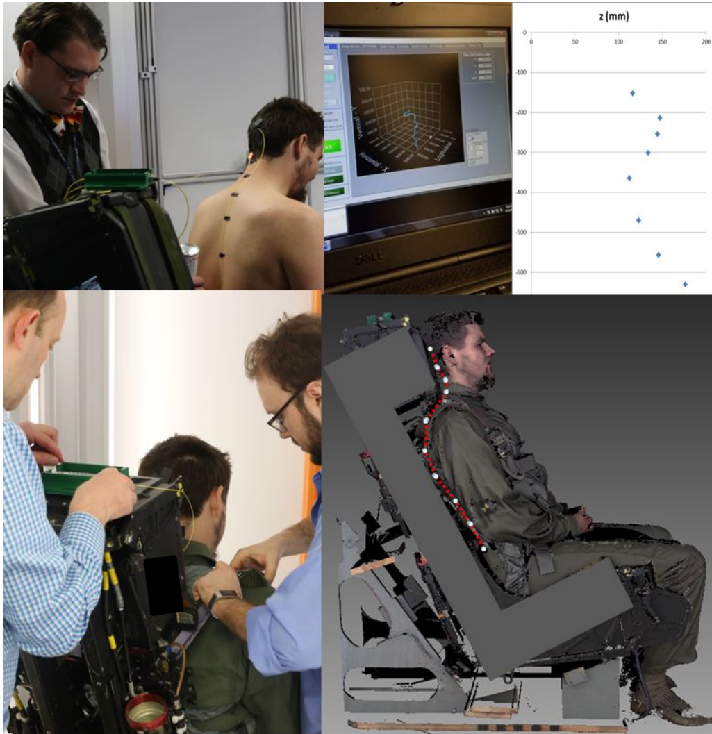
Figure 16. Implementation of Luna system to capture initial posture. Shown in the upper left corner, the subject is “fit” with the Luna system, identifying RAMSIS joint locations using the “cold touch” method. Shown in the upper right corner, the Luna positioning system is displayed in real time. In the lower left corner, the coordinate reference box is mounted to the ejection seat with the subject both encumbered and restrained. Shown in the right corner is the VITUS 3D scan of the subject in the ejections seat with the Luna position data aligned using the coordinate reference box.
