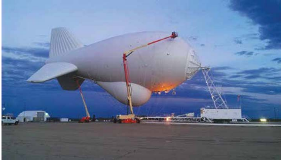
Figure 8. TARS blimps carry a radar payload used to monitor the low-altitude approaches to the U.S. border 263
