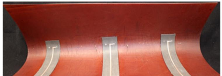
Fig. 5 Fabricated model of curved composite SEVA2 with 3 elements.
