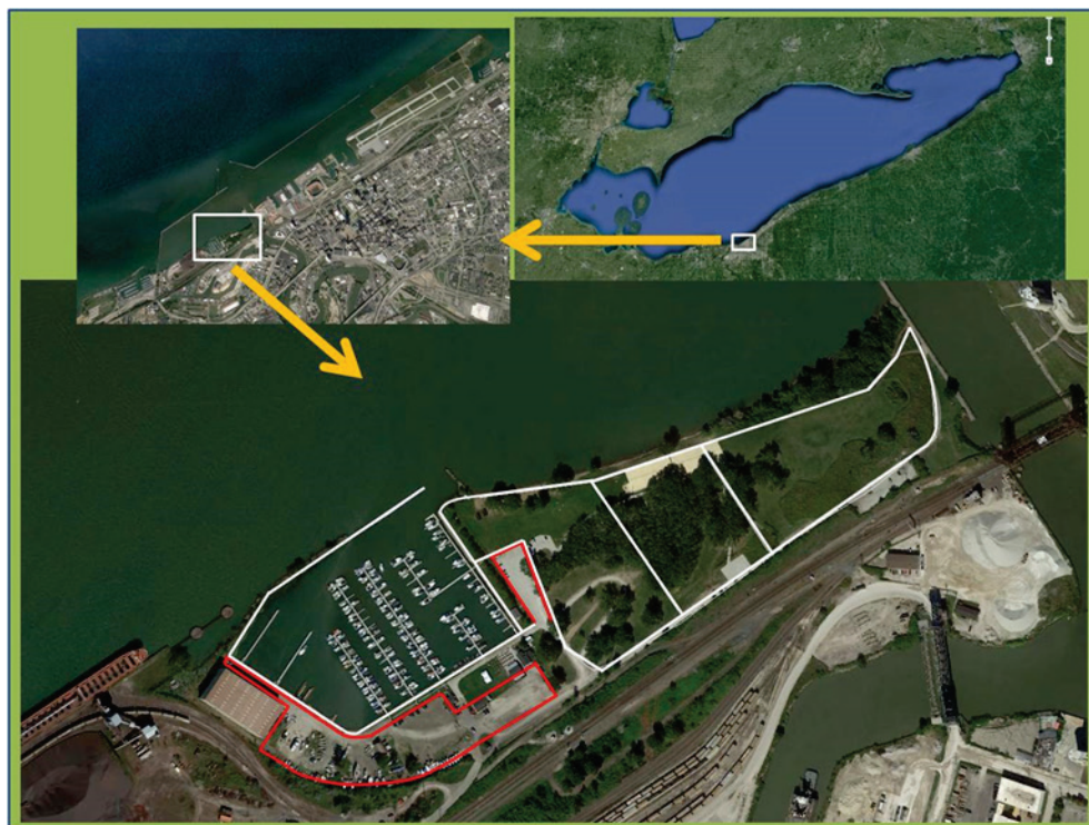
Figure 2. Map of model marina/park development. Walkways are indicated by white lines and paved parking and marina work areas are roughly outlined in red. All docks are to be rebuilt using the current layout. Walkways, paved areas, and docks are to be constructed using photocatalytic cement. Source: "Cleveland Harbor." 41° 28'55.30" N 81° 39'32.99" W. Google Earth. April 18, 2016.
