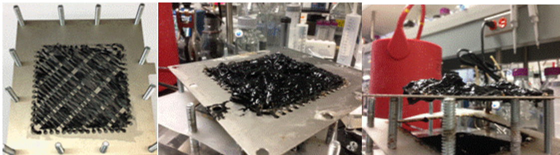
Figure 42. Photos of anode fibers: i) initial (left) and ii) after 12-day HRT at high pH (right).
