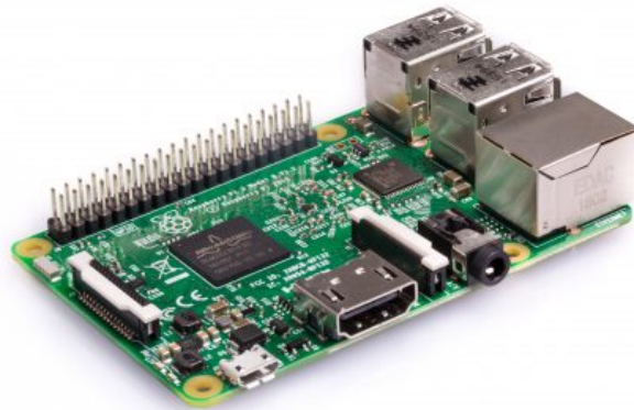
Figure 8. Raspberry Pi 3 Model B. Source: Raspberry Pi Foundation (n.d.)
