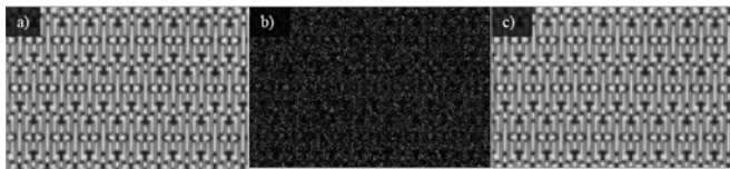
Fig. 14. a) Intel Skylake 14nm processor delayed to M0 on a Plasma FIB. b) simulated image of a) with 20% of the scan data (5X faster!). c) Recovered image using Bayesian Process Factor Analysis.
