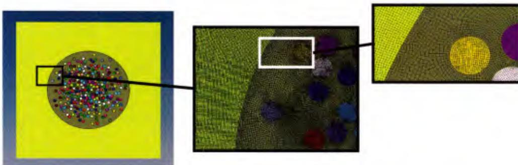
Figure 6: The re-meshed sample showing the different fibers, the surrounding matrix, and the effective composite around the RVE.
