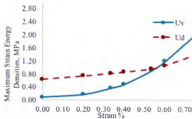
**Figure 3: Variations of maximum dilatation energy density ( $U_v$ ) and distortion energy density ( $U_d$ ) in the RVE realization shown in Figure 2 (circular void) with the applied transverse strain.**
