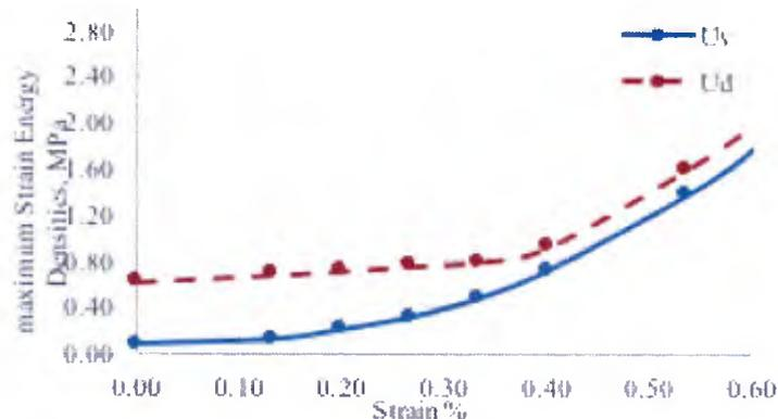
**Figure 4: Variations of maximum dilatation energy density ( $U_v$ ) and distortion energy density ( $U_d$ ) in the RVE realization shown in Figure 2 (elliptical void) with the applied transverse strain.**
