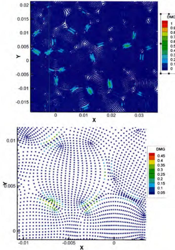
**Figure 7: Top: the damage index over a set of fibers showing that fiber-bonds that cross between two fibers have been eliminated. Bottom: a zoomed-in figure around one fiber.**
