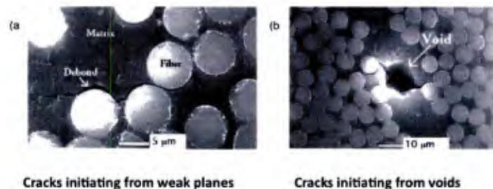
Figure 1. Cracks initiation without matrix voids (a) and with matrix voids (b).
