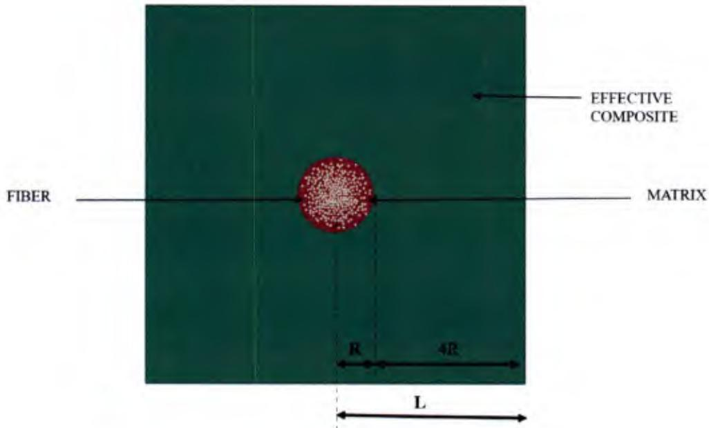
Figure 5: The RVE from the SDM model (provided by Prof. Talreja's group) used in the peridynamic model. To reduce computational costs, a smaller amount of effective composite material is used by transferring the appropriate boundary conditions to near the fiber bundle region. The new sample is re-meshed to ensure a more uniform size of elements (which will result in a more uniform size of nodal areas for peridynamic nodes. This is shown in Fig. 6.
