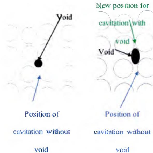
**Figure 2.** Figure shows regions of RVE realizations analyzed with matrix voids inserted. Left: a circular void and Right: an elliptical void placed with its major axis normal to the load direction (horizontal). The position of points where brittle cavitation occurs is indicated. As shown, this position shifts to another location when an elliptical crack is present.
