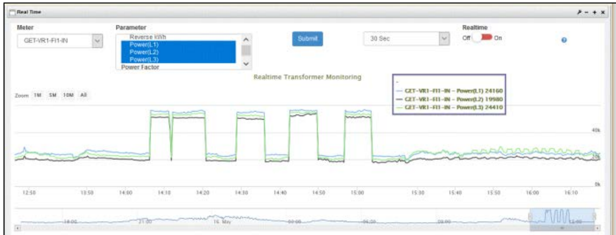
Figure 30. Power Monitoring Mode Output for 100 kVA High Variation Load Testing May 16, 2017
