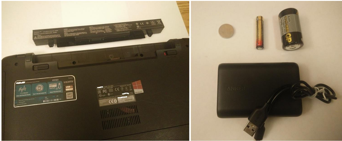
Figure 7. Smart Battery in a Laptop (left). Standalone Bare-Bones Batteries (right).
