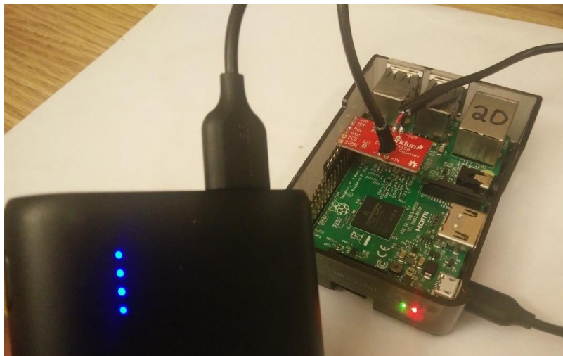
Figure 35. Actual Fitting of LTC 4150 into Raspberry Pi 3B with Anker PowerCore 10000
