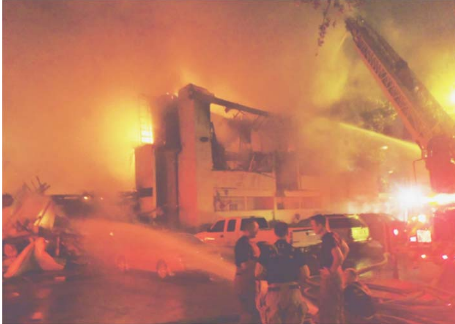
Figure 15. Elevated Master Stream in Operation on May 20, 2013 332
