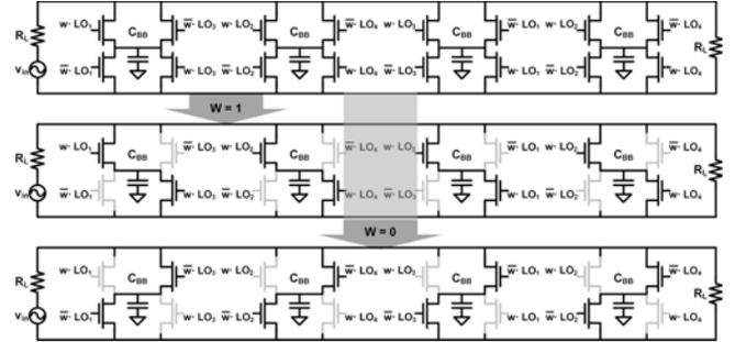
Figure 3. Model of a shunt code selective filter based on the linear, time-variant  $N$ -path circuit.
