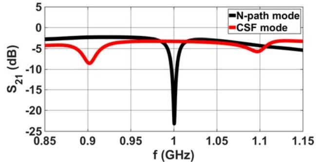
Figure 7. Frequency response of the CSF in the presence of a CW input when 1) the switches are modulated as a period  $1/N$  clock sequence (dashed line/black) and 2) the switches are modulated with a PN sequence.
