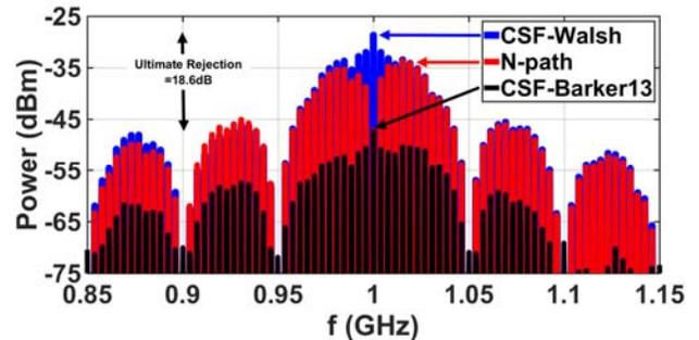
Figure 8. Comparison of the filter rejection for different code states illustrating the potential for wideband signal rejection.
