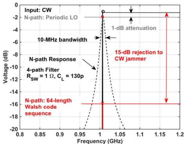
Figure 5. Frequency response of the CSF in the presence of a CW input when 1) the switches are modulated as a period  $1/N$  clock (dashed line/black) and 2) the switches are modulated with a PN sequence.
