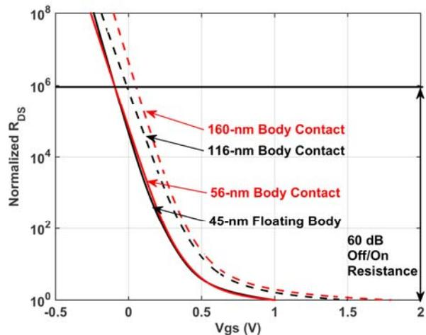
Figure 6. ON resistance of n-FET devices in SOI CMOS for different device configurations at different channel lengths.
