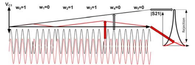
Figure 4. Illustration of the code-selective filter as distinguished from an  $N$ -path filter. Orthogonal codes are integrated to zero charge on the capacitor reducing the impedance that is seen by the RF signal.
