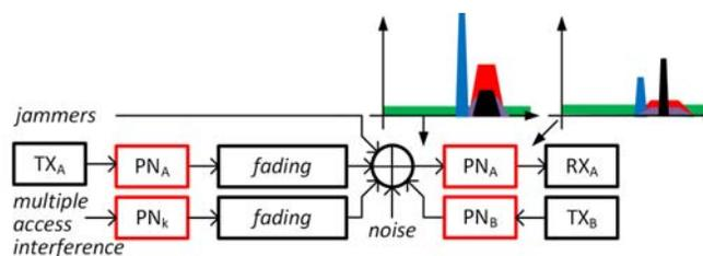
Figure 1. Channel model for direct-sequence spread spectrum for full-duplex communication. The desired signal (shown in black) is selected in the receiver while orthogonal signals (shown in red) and jammers (shown in blue) are rejected.
