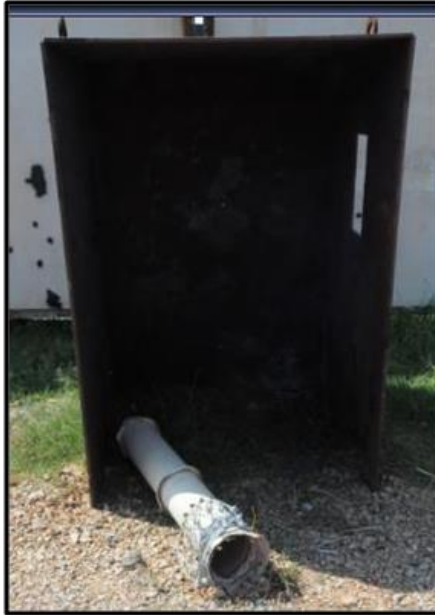
Figure 38 Container propelled into steel wall
