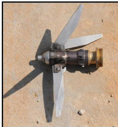
Figure 42 Recovered unarmed fuze and fin assembly (x-rayed)
