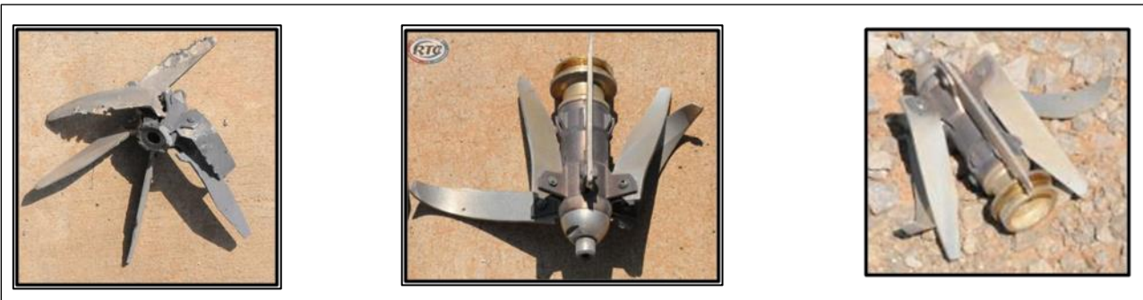
Figure 37 Recovered fin and fuze assemblies
