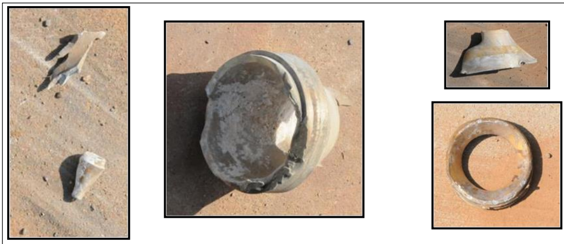
Figure 44 Recovered warhead fragments
