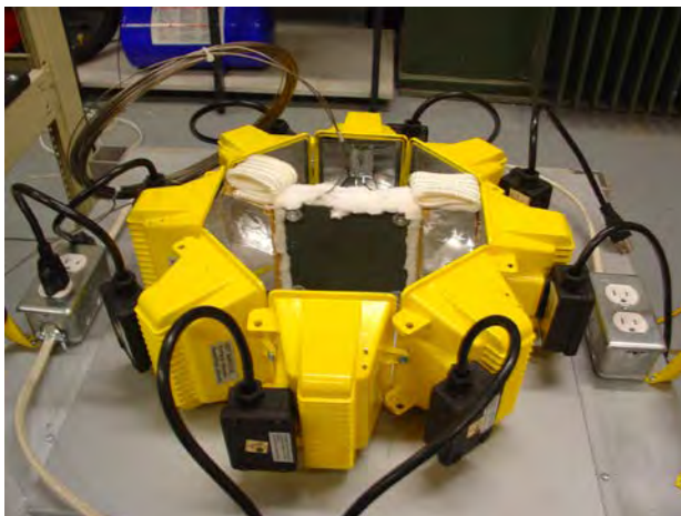
Figure 9. Differential Flame Thermometer (DFT) being tested in a radiant chamber, and resulting temperature versus time on the inside face of the DFT.
