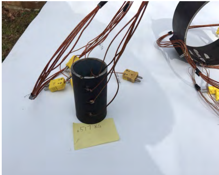
Figure 6. Calorimeter for calibrating heat flux and showing uniformity of temperature and heat flux. Three axial stations were monitored on both surfaces of the calorimeter.
