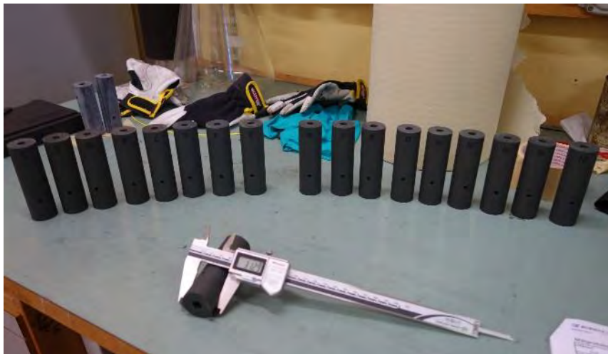
Figure 8 Photo of extruded propellant grains for ballistic testing
