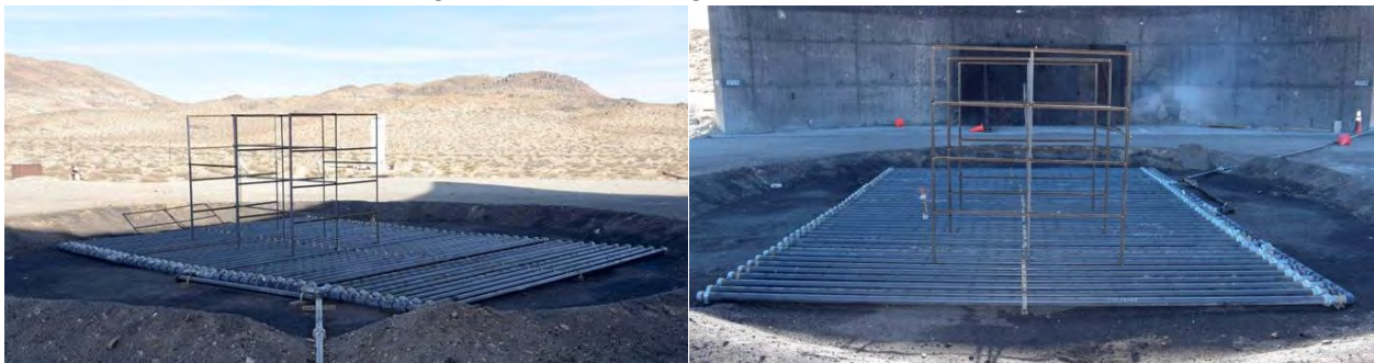
Figure 1. 4.6 m by 6.1 m Propane Burner Built at China Lake
