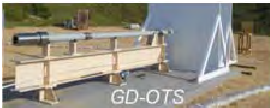
Figure 2. Typical fragment impact test setup
