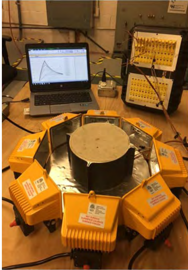
Figure 1. Radiant chamber set up for testing a segment of a rocket motor with inert propellant. The test item has thermocouples to measure the temperature along three thermal paths to the propellant. Temperatures are measured on the outer surface of the motor, the inner surface between the motor and insulation, and between the insulation and the propellant. The computer screen shows the data traces which were viewed in real time as the test evolved. The power was turned off when the motor would have cooked off, which is when the traces turn down and the motor cools.
