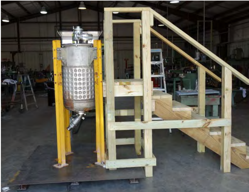
Lacquer Preparation Vessel
