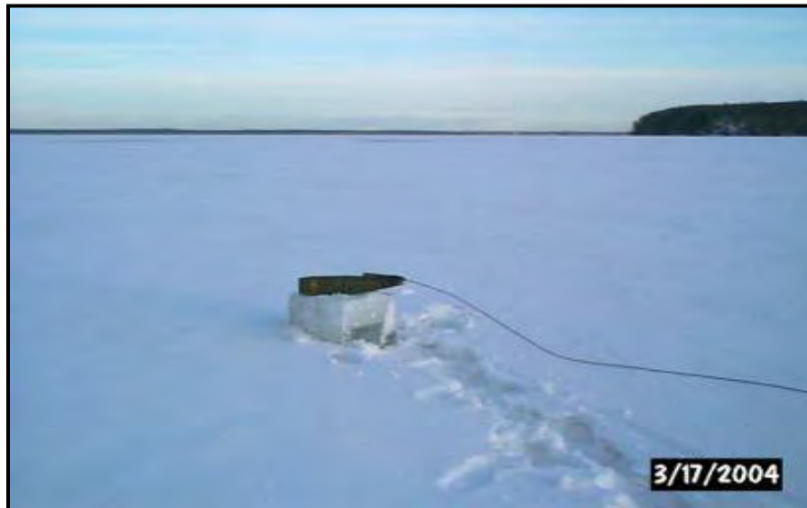
Figure 1: A munition on a block of ice ready for detonation (past test, not the current munition)
