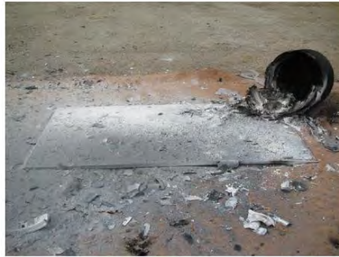
Figure 8 : witness plate after the test
