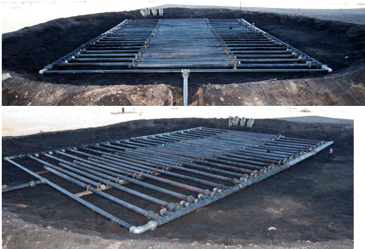
Figure 2. Modified 4.6 m by 6.1 m Burner
