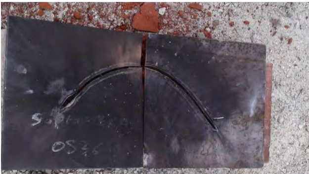
Picture 12: Cut steel plate after ignition
