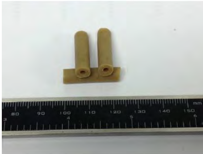
Figure 3: BN-RPD380 (US Patent Pending) Single Perf grains used in erosion testing
