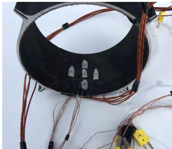
Figure 14. Interior instrumentation showing thermocouples to measure the temperature at the interface between the insulation and propellant.
