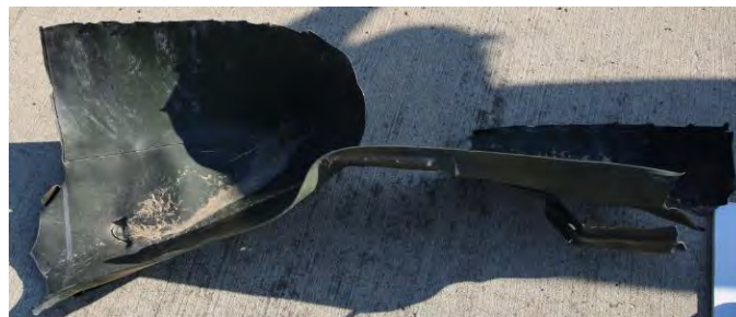
Figure 8: Ammo can post-test, completely blown open
