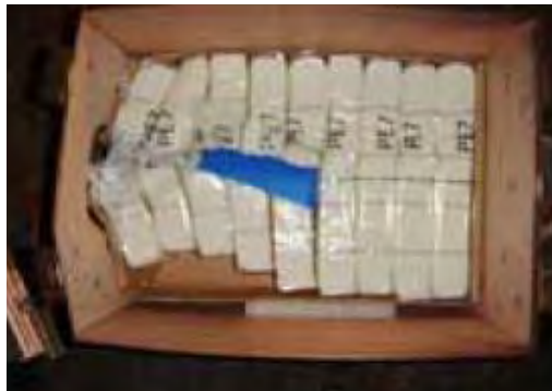
Picture 7: Hexomax after the bullet impact
