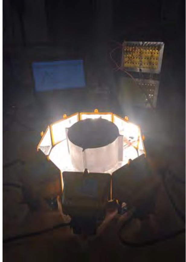
Figure 1. Radiant chamber set up for testing a segment of a rocket motor with inert propellant. The test item has thermocouples to measure the temperature along three thermal paths to the propellant. Temperatures are measured on the outer surface of the motor, the inner surface between the motor and insulation, and between the insulation and the propellant. The computer screen shows the data traces which were viewed in real time as the test evolved. The power was turned off when the motor would have cooked off, which is when the traces turn down and the motor cools.
