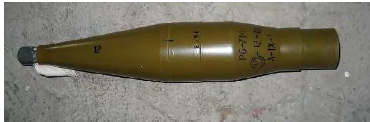
Figure 3 : RPG-7 Shaped charge used for the trial
