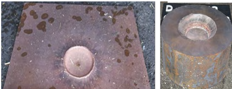
Fig. 3: Cu witness plate of configuration 2 (left) and steel block of configuration 3 without Cu sample (right) after the firings.
