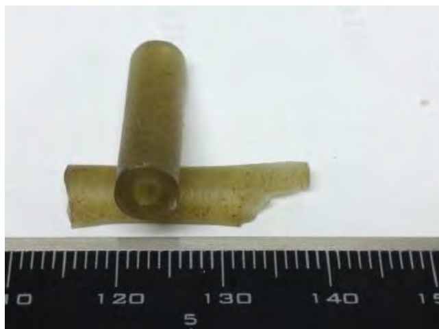
Figure 2: RPD380 without BN - Single Perf grain used in erosion testing
