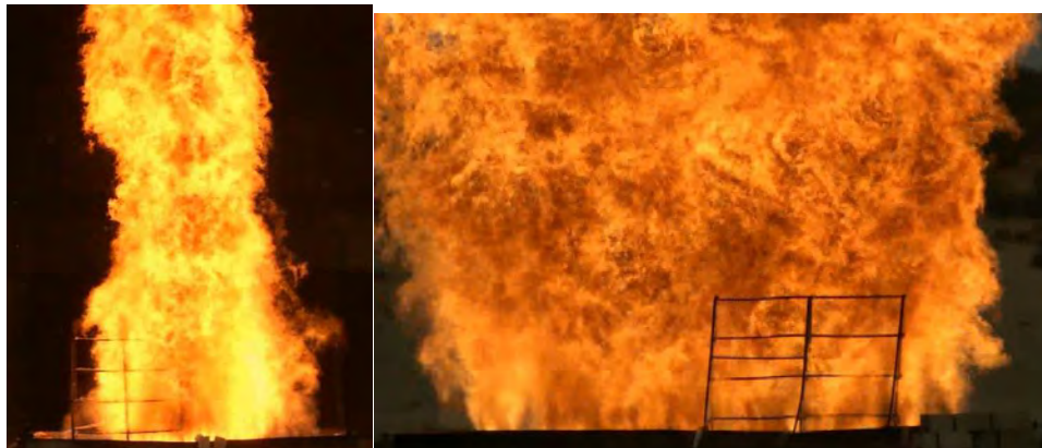
Figure 3. Qualitative Flame Structure for Modified 4.6 m by 6.1 m Propane Burner
