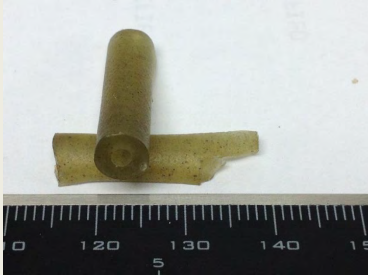
Figure 1: RPD380 w/o BN - Single Perf grain used in erosion testing
