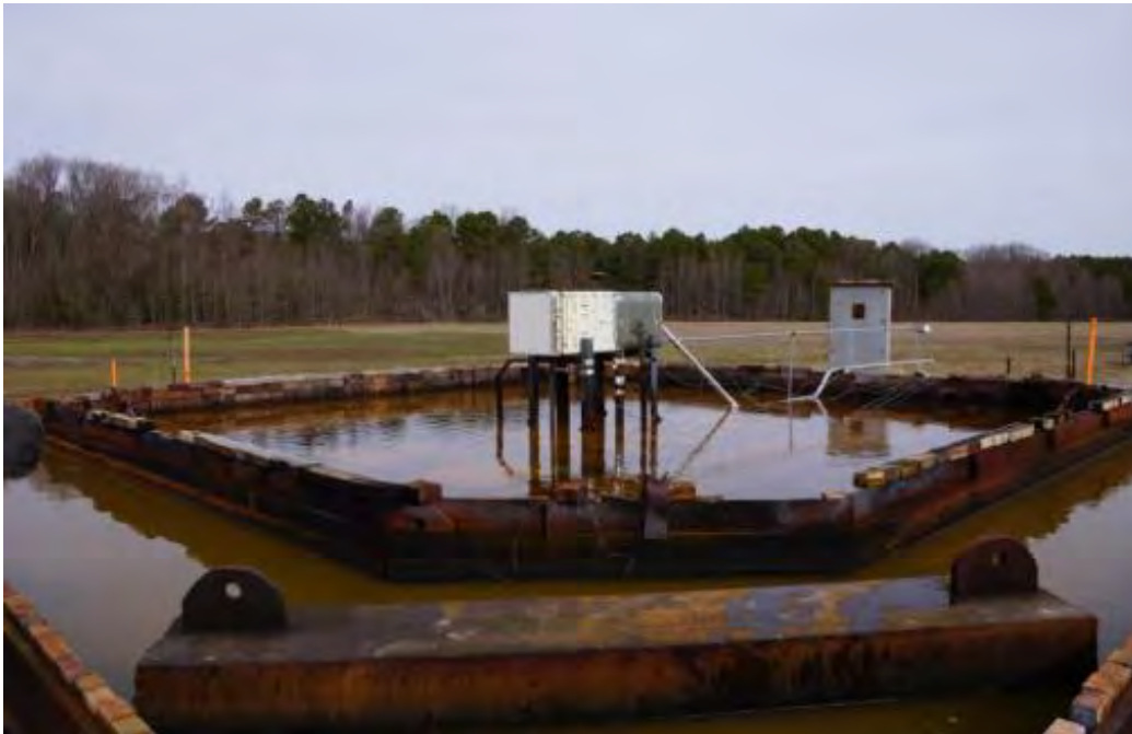
Figure 1. Steel and carbon fiber canisters in Dahlgren fast cook-off pit.
