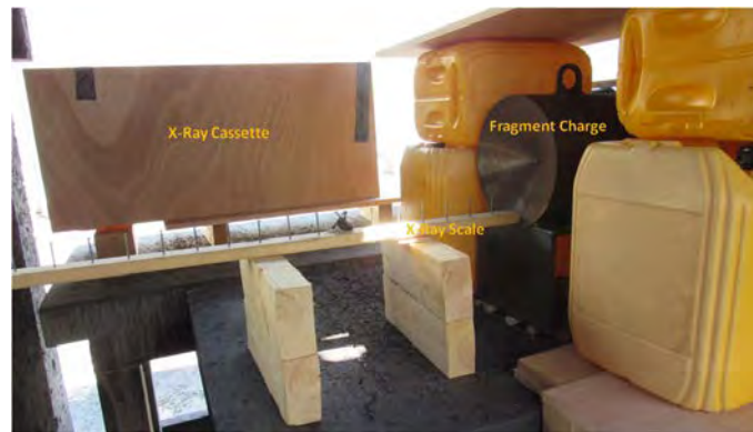
Figure 4 – 1830 m/s charge test setup
