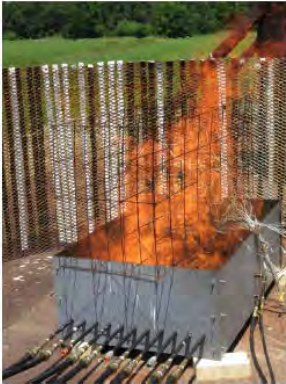
Dahlgren .6 x 1.2 m propane demo burner
