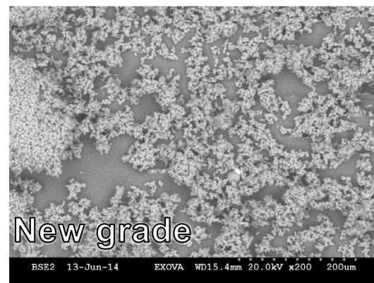
Fig 13. FOX 7 X-fin 140528.2, 200x magnification.
