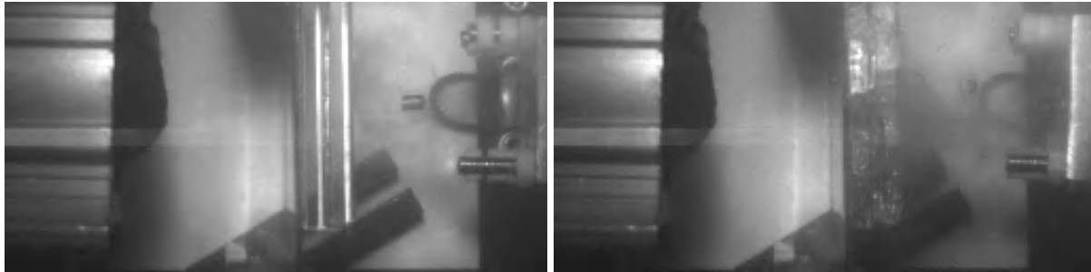
Figure 6: Left Typical toughened glass laminate target before impact, projectile approaching from right hand side. Right Target after impact, fracture to glass evident and fragment has ricocheted at 45 m/s.
