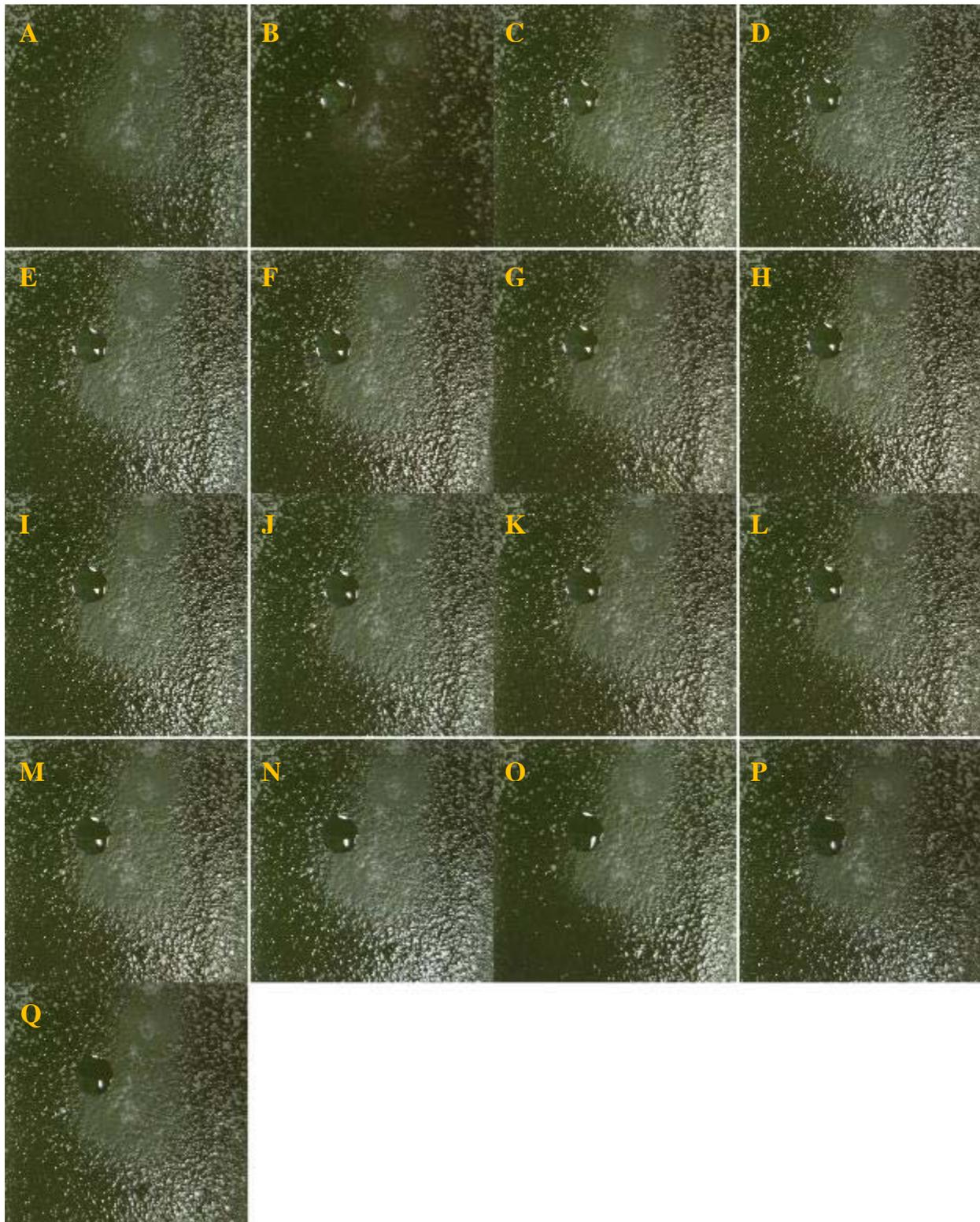
Fig. A12 — DMMP on the Corin 0578 coating. Images of a coupon before application (A) and at 0 (B), 0.5 (C), 1 (D), 1.5 (E), 2 (F), 2.5 (G), 3 (H), 3.5 (I), 4 (J), 4.5 (K), 5 (L), 10 (M), 15 (N), 20 (O), 25 (P), and 30 (Q) min following application of the target.
