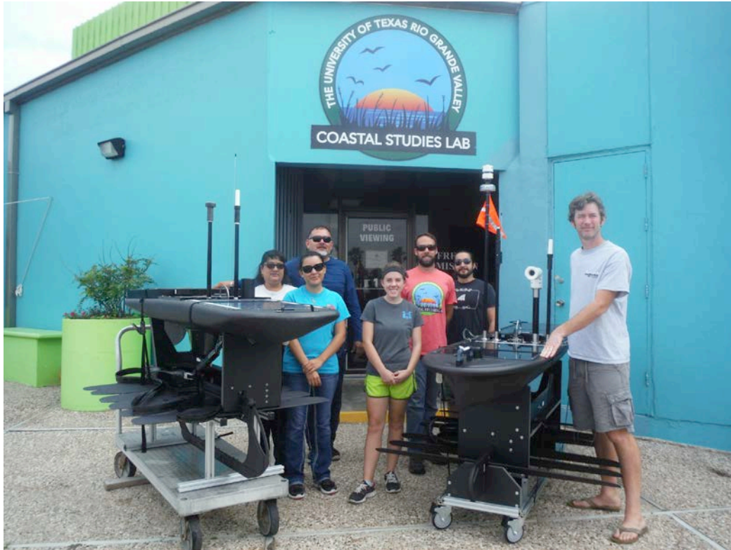
Figure 1. The Liquid Robotics Wave Glider SV3 procured in this project is shown on the right and consists of a surface float and a subsurface glider/propulsor. The glider/propulsor can passively extract power for propulsion from ocean waves. Solar panels and batteries in the surface float provide power for instruments and control computers. The bottom of the float and the wings of the glider/propulsor will be used as biofouling test surfaces.
