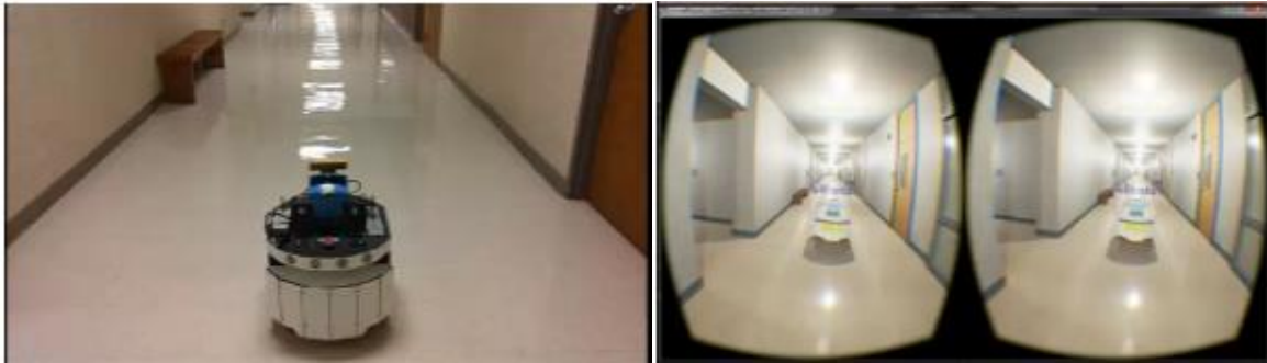
Figure 5. The robot operation with VETO: Left- PatrolBot in the real world. Right- the PatrolBot as observed and operated in the Virtual World through Oculus Rift HMD (Head Mounted Display).
