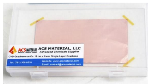
Figure 20. CVD-grown graphene on Copper foil purchased from ACS material
