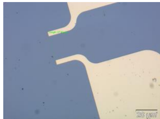
Figure 8. Optical images of the metal contacts on graphene.
