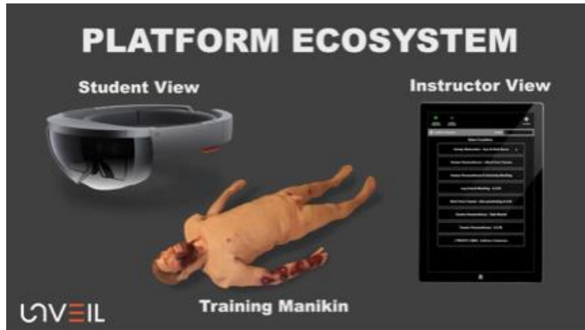
Figure 1. MART platform ecosystem, including an AR headset, smart manikin, and instructor tablet app
