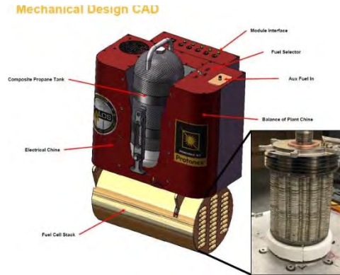
TALOS Solid Oxide Fuel Cell Power & Energy
