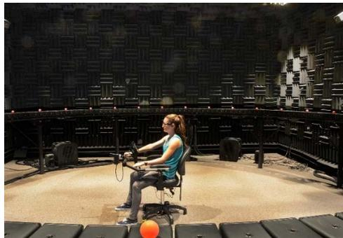
**Fig. 3 Loudspeaker configuration in the dome room. Method 2 testing incorporates 36 loudspeakers spaced at even intervals of 10°, beginning at 5° and continuing to 355°.**
