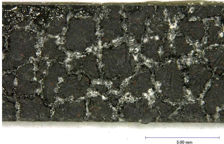
Figure 39. Optical Photograph of a Tension-Tested A500 C/SiC Sample (#8) After 1500 Burner Rig Cycles and 120 Hours Salt Fog Exposure
