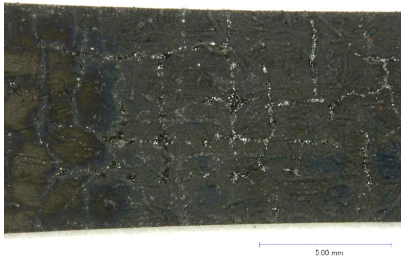
Figure 33. Optical Photograph of a Tension-Tested A500 C/SiC Sample (#13) After 600 Burner Rig Cycles and 48 Hours Salt Fog Exposure
