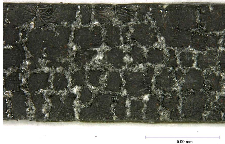
Figure 52. Optical Photograph of the Surface of the Gage Section of a A500 C/SiC Fatigue Specimen Pre-conditioned (1 Hz, 150 MPa, 24°C, 1000 Cycles) After 1500 Burner Rig Cycles Plus Salt Fog Exposure
