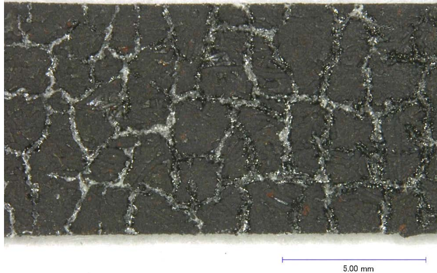
Figure 35. Optical Photograph of a Tension-Tested A500 C/SiC Sample (#4) After 900 Burner Rig Cycles and 72 Hours Salt Fog Exposure
