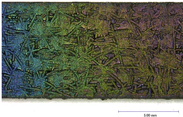
Figure 48. Optical Photograph Of The Surface Of The Gage Section of A500 C/SiC Specimen After 1500 Burner Rig Cycles and No Salt Fog Exposure
