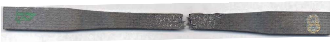
Figure 49. Optical PhotographOf A Tension Tested A500 C/SiC Specimen After 1500 Burner Rig Cycles Plus Salt Fog Exposure
