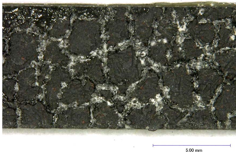
Figure 50. Optical Photograph Of The Surface Of The Gage Section of A500 C/SiC After 1500 Burner Rig Cycles Plus Salt Fog Exposure
