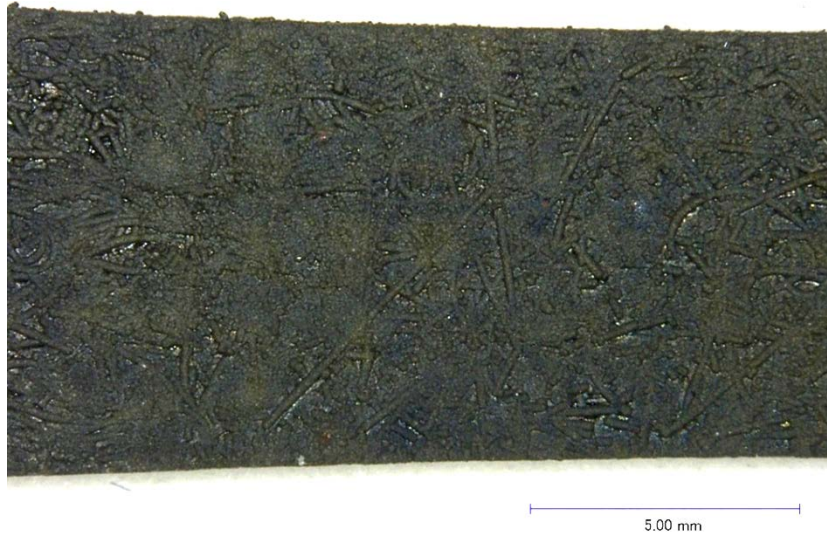
Figure 31. Optical Photograph Of A Tension-Tested A500 C/SiC Sample (#3) After 300 Burner Rig Cycles and 24 Hours Salt Fog Exposure
