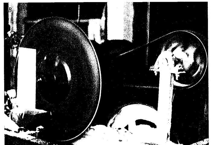
6. Modern machine-made shingles are sawn. Shown are: (photo A) Eastern White Pine quarter split shingle block on equalizer saw being trimmed to parallel the ends; and (photo B) the restored 19th-century shingle mill saw cutting tapered flitches or shingles. The thickness and taper can be precisely controlled. Photo: Steve Ruscio, The Shingle Mill.
