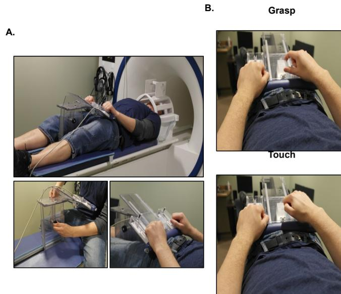
*Figure 2. MRI-compatible system for investigating neural control of manual reaching and grasping movements.*
