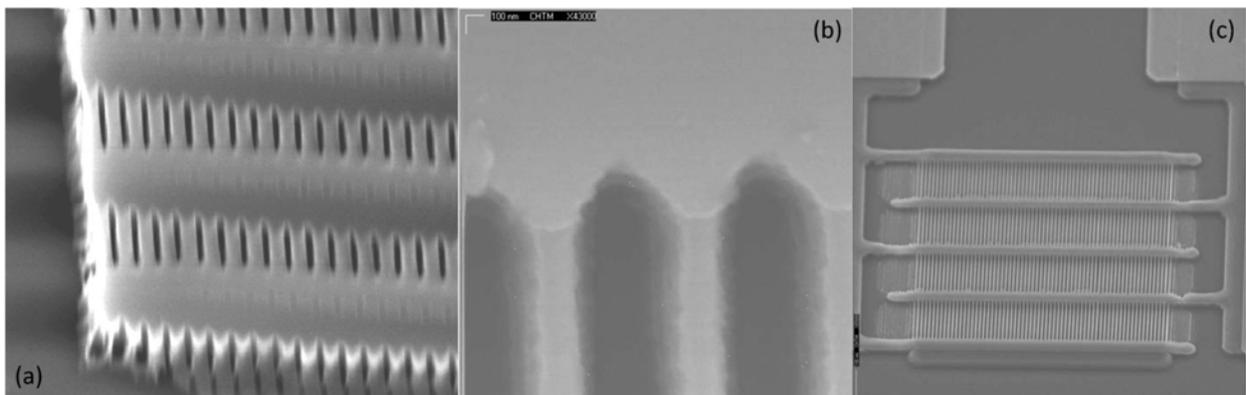
**Figure 3. SEM images of (a) pre-oxidized Si mesa configuration with precursors to wall structures in the active region in-between planar un-textured regions where the metal contacts will be deposited; (b) planar un-textured Si where thermally grown oxide was removed for metal contact deposition connecting walls; (c) fully fabricated wall device with interdigitated electrodes.**
