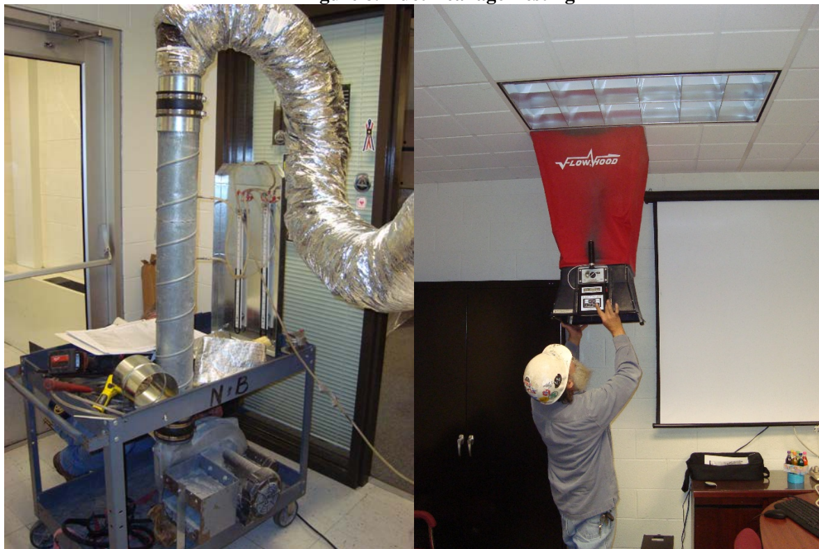
Figure 8. Duct Leakage Testing
