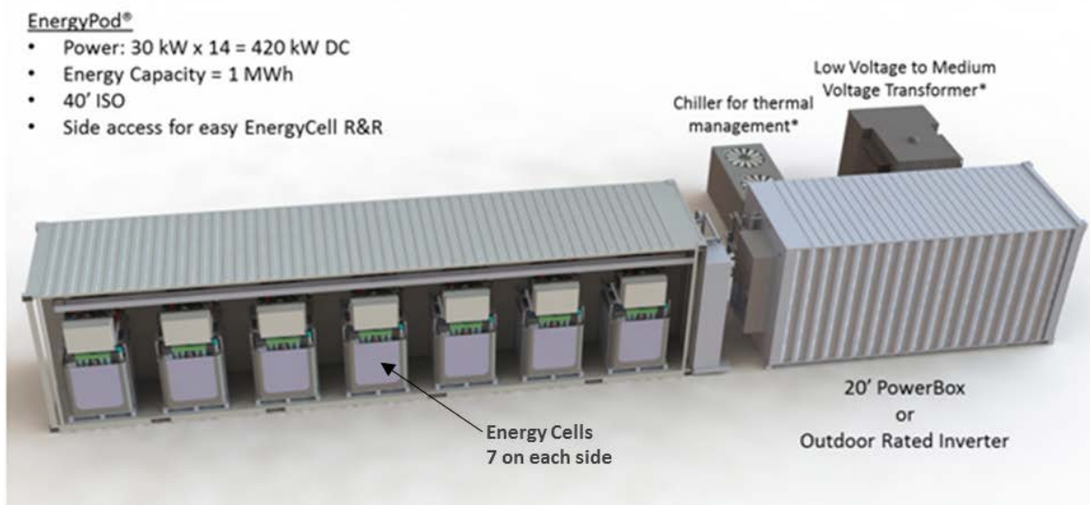
Figure 6. Illustration of Primus' ESS, Complete with EnergyPod (Zn/Br EnergyCells), PowerBox (power electronics), and Thermal Management.
