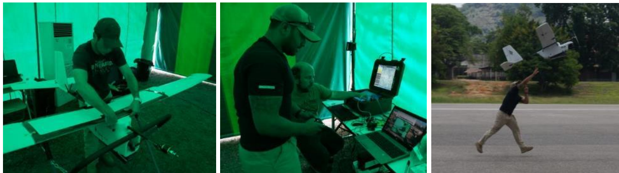
Figure 35: Talon 120LE Assembly and Preflight checks (Left and Center) and Talon 120LE Hand Launch (Right)
