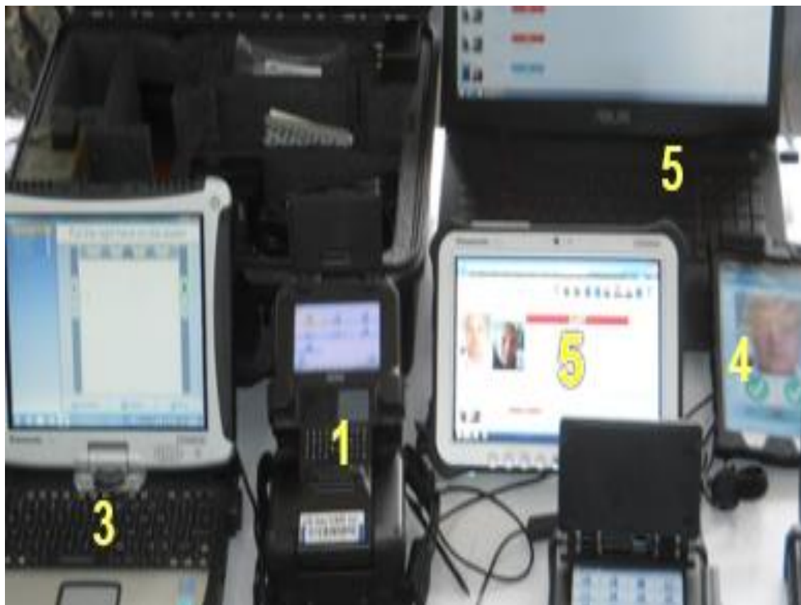
Figure 57: Actual gear onsite at CV15 (1) SEEK II; (2) SEEK Avenger; (3) Guardian Jump Kit laptop computer, fingerprint scanner, iris scanner, and mug shot camera; (4) SRI Galaxy Identification Pro Tablet; (5) ASUS server and Toughbook server remote screen
