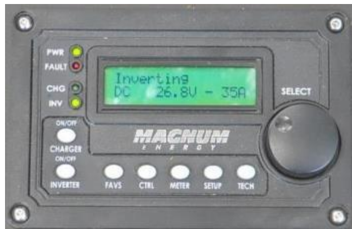
Figure 33: STAESS LCD Control Panel
