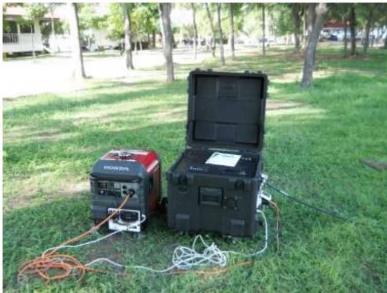
Figure 21: Schematics or diagrams can be printed the inside lid of the Smart PPS module
