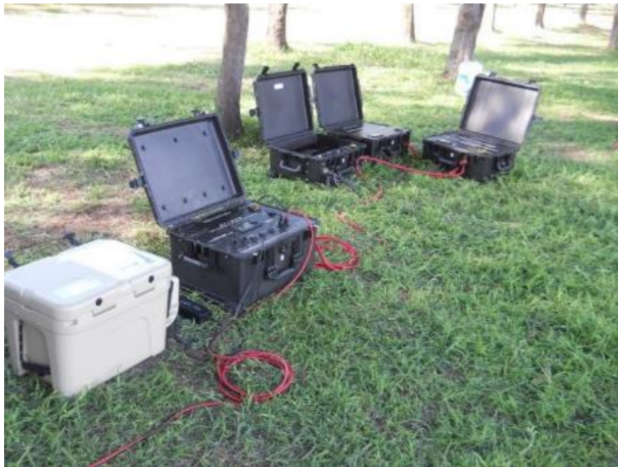
Figure 44: STAESS providing electricity to a thermoelectric cooler.
