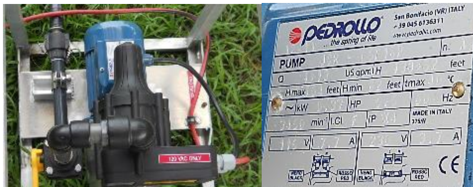
Figure 54: Label on the pump module indicating the use of 120 VAC electricity only (Left), Pump nameplate showing that the pump motor can be wired for either 120 VAC or 240 VAC electricity (Right)
