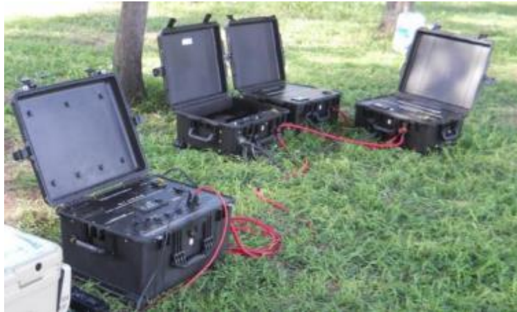
Figure 36: Battery banks, charge controller modules, inverter with cases open
