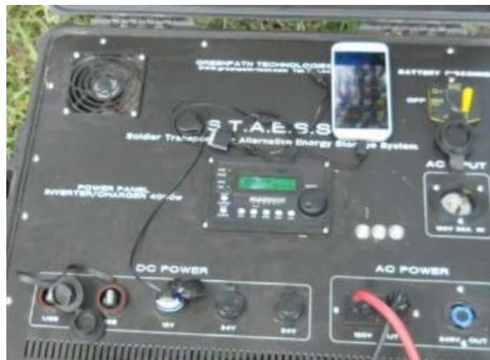
Figure 37: USB chargers did not work. A USB-cigarette adaptor on the 12VDC receptacle to had to be used to charge cell phone
