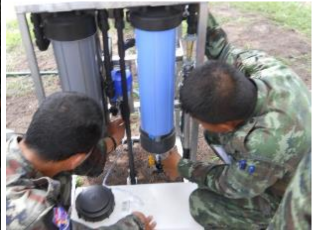
Figure 55: RTAF personnel adding chlorine to First Response 5000
