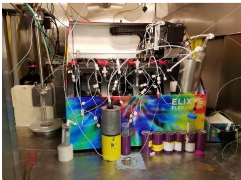
Figure 3. Elixys synthesis unit that has been programmed to prepare SFB and label the AH-TG97 precursors.
