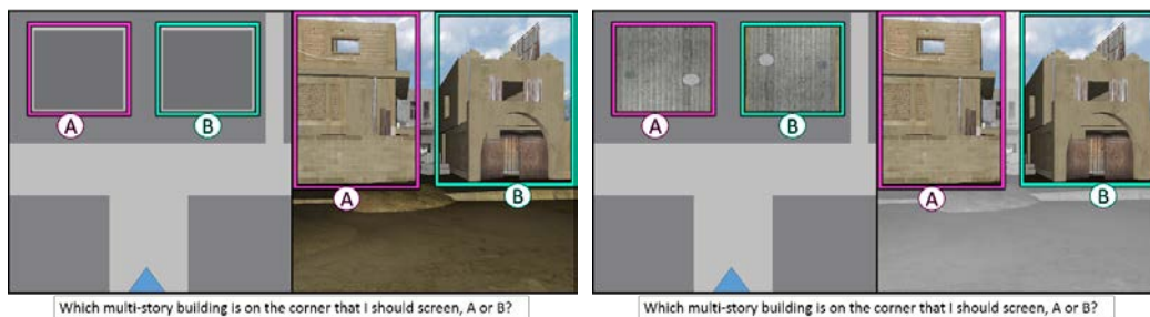
Fig. 10 Two images representing the robot's building-identification-query display formats in the MMI; image on the left has highlighted boxes around the buildings (Building A) while the image on the right has highlighted boxes around the buildings with modifications to the scene and aerial images (Building B)
