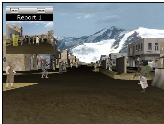
Fig. 5 Image represents an alternative use of the virtual MMI, whereby status updates can be requested from the robot
