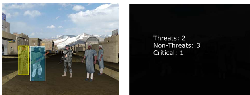
Fig. 14 Robot's report shows unsafe immediate environment; (left) in image report a critical threat is bounded in blue box while (right) the text report counts the number of critical threats
