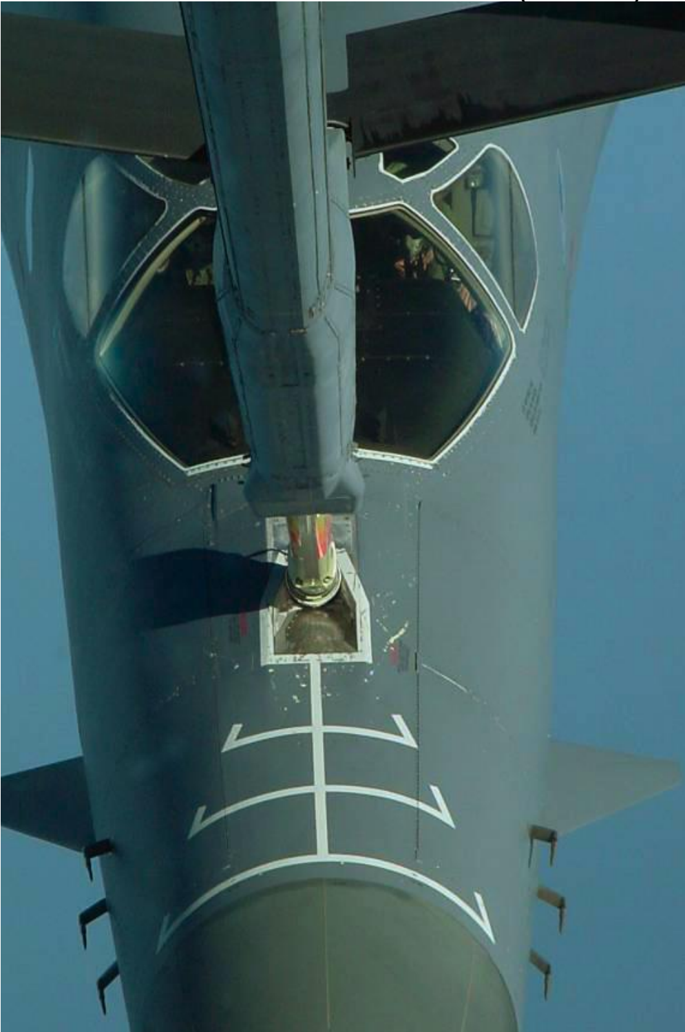
Figure 12.3.2.2 Triple Bar Receptacle Markings
