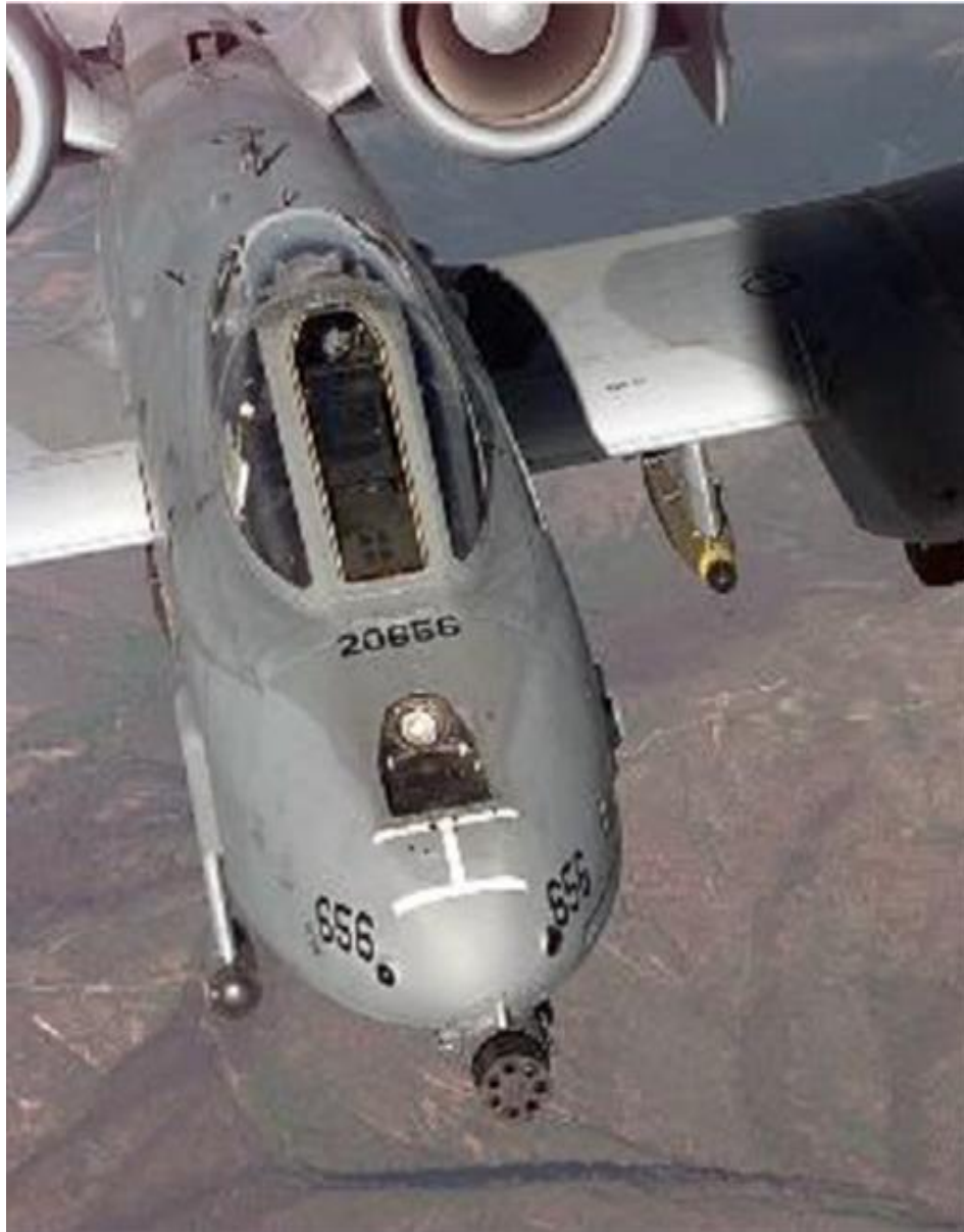
Figure 12.3.2.11 Two-bar Receptacle Markings
