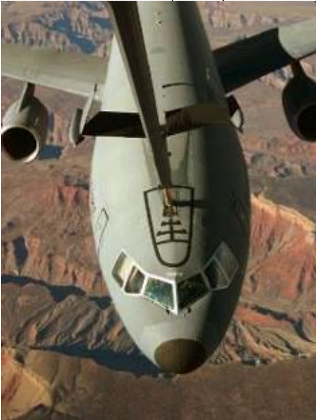
Figure 12.3.2.7 Triple Bar UARRSI Markings - Camouflaged
