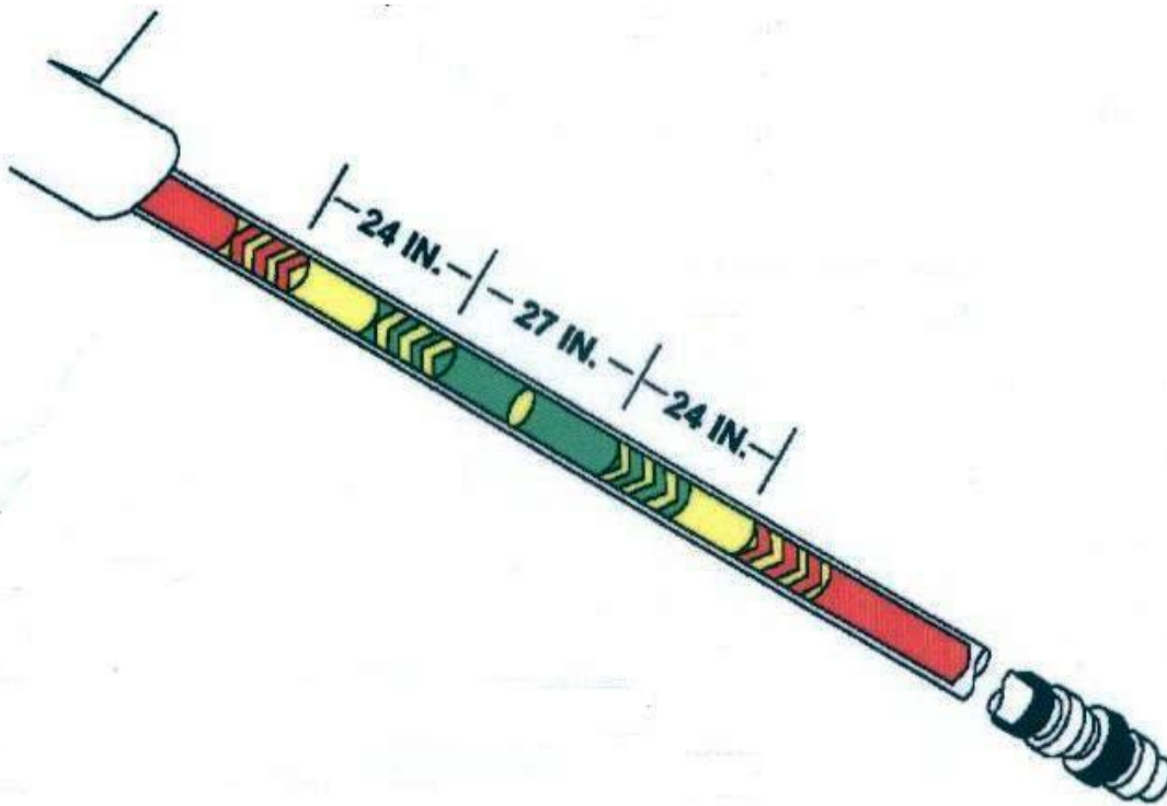
Figure 12.2.4.2 Boom Telescopic Tube Markings
