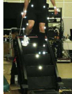
Figure 9: Stair Descent Speed-adapting Stairmill. The resistive alternator of a commercially available stairmill has been replaced with a powered motor for reverse direction operation. Motion capture during stair ambulation test using sensorized boot and vibrotactile stimulation thigh strap (right).
