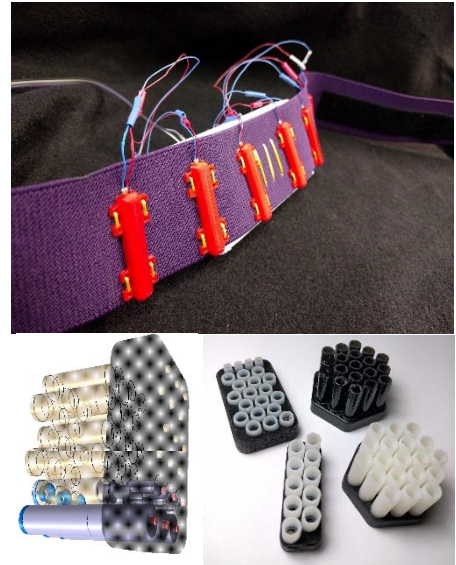
Figure 5: Above: Array of piezoelectric vibrotactors, under custom skin interface enclosures. The strap affixes the array to the thigh, outside of the socket. Below: High-resolution arrays of factors.
