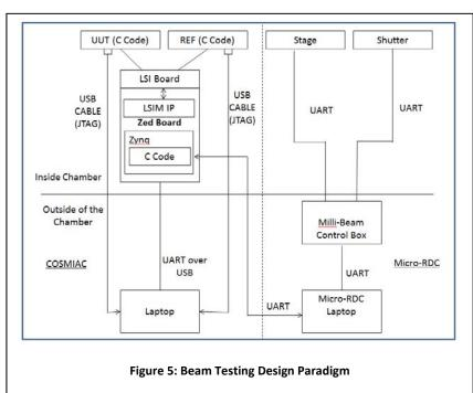
hardware and software configuration that was utilized for beam testing of the MSP-430 microcontrollers.
