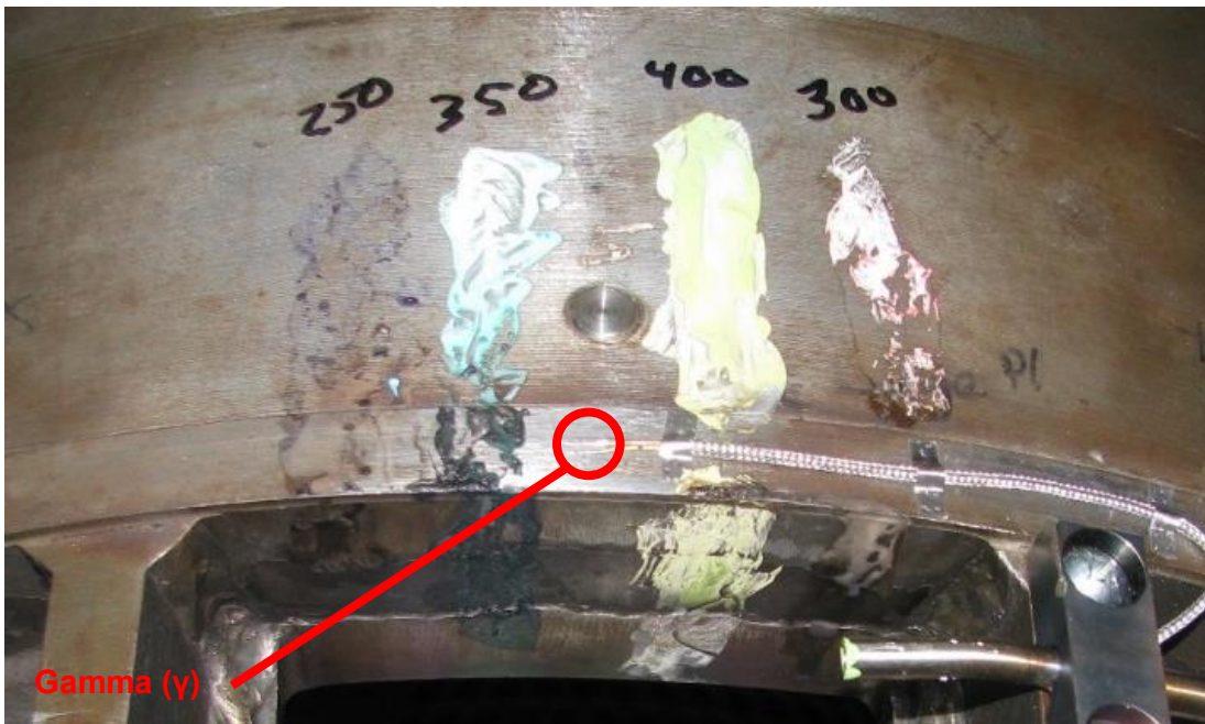
Figure 9. Temperature Melting Paint After Test Program
