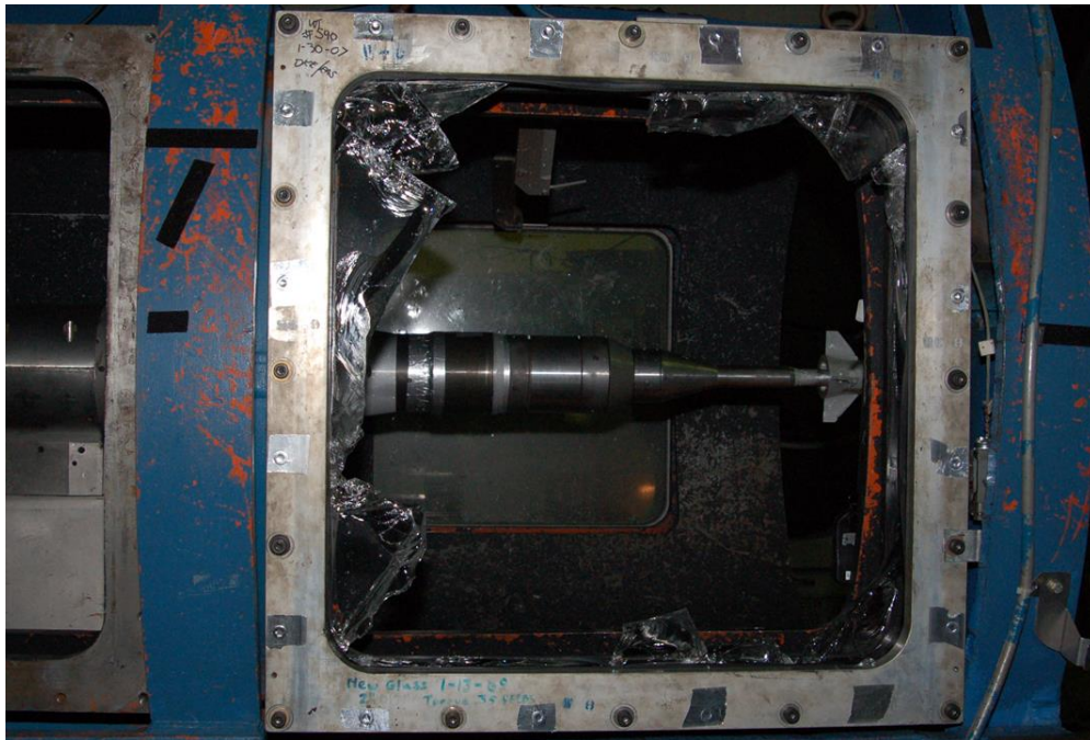
Figure 3. Broken Test Cell Window
