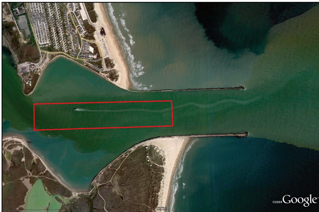
Figure 8-16. Location (in red) of the deepened portion of the channel for the In-Channel Sediment Trap Alternative (from Google Earth https://www.google.com/earth/ ).
