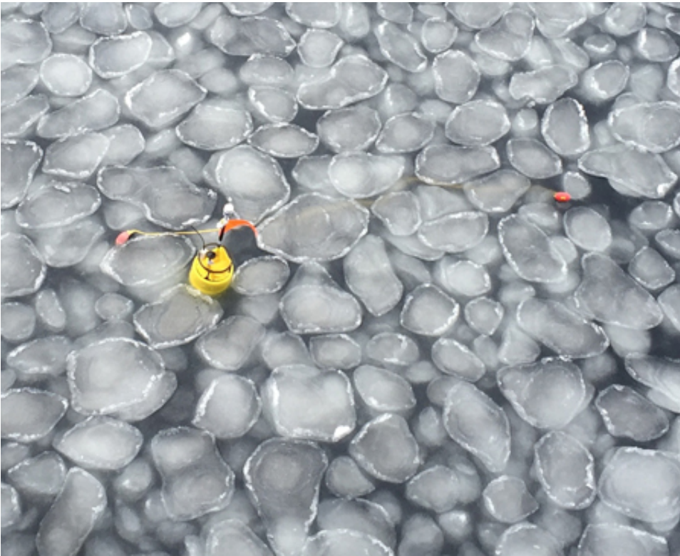
Fig. 2. A Surface Wave Instrument Float with Tracking (SWIFT) buoy measures waves in pancake ice. Credit: Benjamin Holt, NASA/JPL-Caltech
