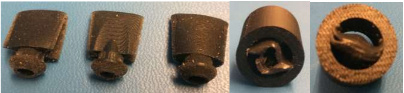
Figure 4 – Three valve prototype designs from the first design iteration (left) a soft valve showing tearing as it opens (middle) and a winged valve not opening (right).
