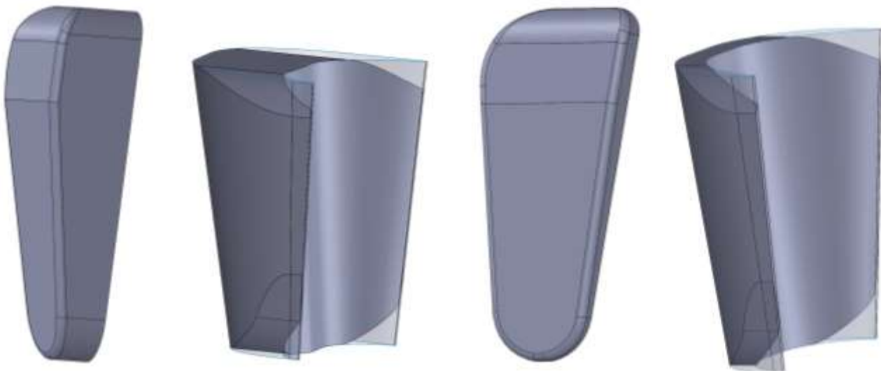
Figure 1 – Solid models of the medial and posterior volume elements 40mm thick (left pair) 11.5mm thick (right pair). The posterior elements (on the right in each pair) display the new curved shape.
