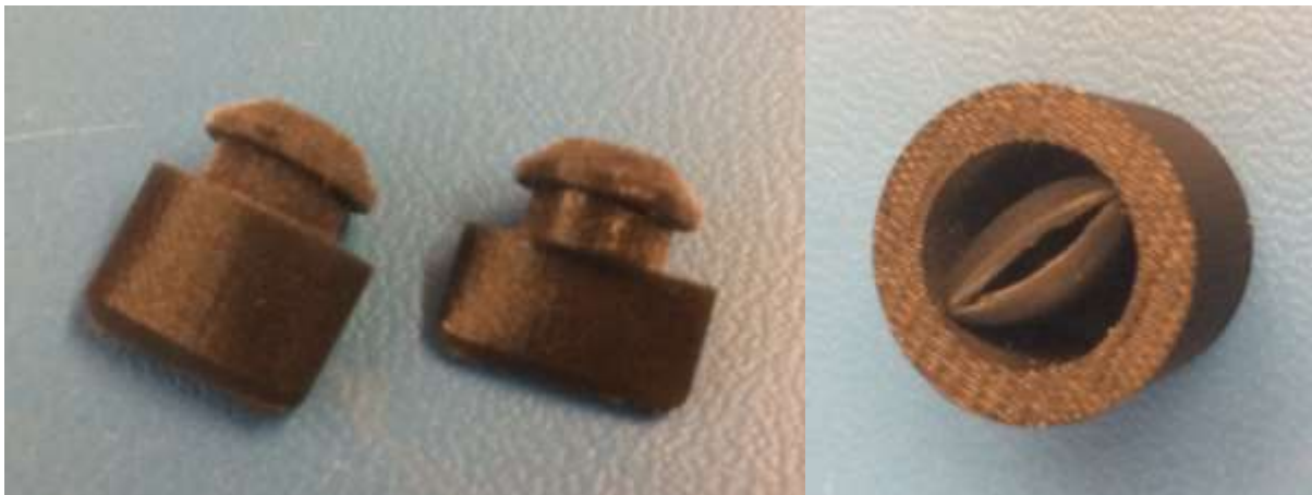
Figure 5 – The most recent valve prototypes (left), the shorter of which is being opened by the cylinder (right)
