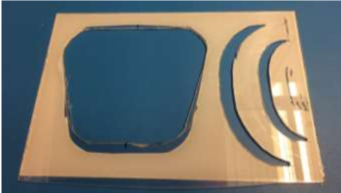
Figure 3 – A template for cutting the distal volume element
