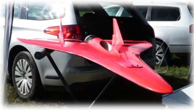
Figure 6. sUAS powered by a Behotec JB-180 turbine engine
