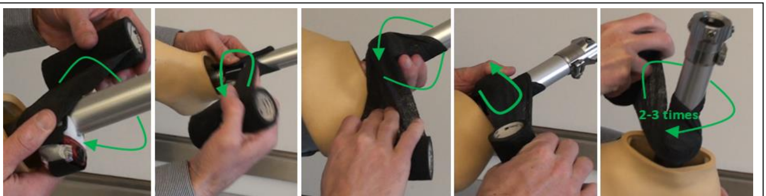
Figure 5: Sequential steps to wrap ankle pylon (left to right). Wrap very tightly in order to secure it. If the ActiGraph rotates about the pylon during the duration of the study, it can affect the quality of the activity data.
