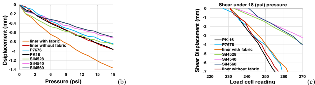
Figure 2: characterize the compression and shear moduli of silicone materials; (a) comparison of displacement-pressure relationships of different materials; (b) comparison of displacement-shear load relationship of different materials.
