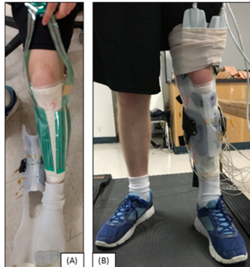
Figure 17. The PTB-AFO Test: (A) The leg of the healthy volunteer is shown covered in a sock with attached F-Socket load sensors; (B) The first iteration of the PTB-AFO on a treadmill with air and F-Socket communication lines leading to a tabletop test setup close by.
