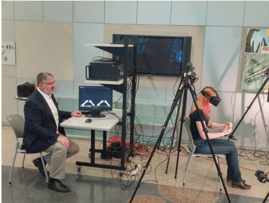
Figure 1 – The infrared motion tracking system. A student is shown wearing the Oculus Rift goggles and infrared hand tracking system. The screen shows the position of the student’s hands captured by tracking systems and displayed to her by the goggles. This demonstration of the real-time hand tracking and virtual reality environment was filmed for use on multiple news programs.
