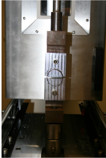
(a) Split ring fixtures and bearing cage mounted
