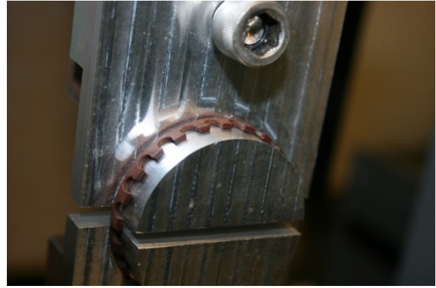
(b) Close up look at the bearing cage mounted on the fixture
