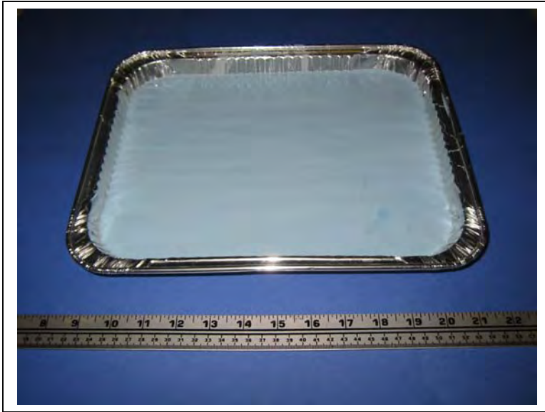
Figure 1a. 3cm thick rectangular slab constructed using GI-1000 RTV and diluent.
